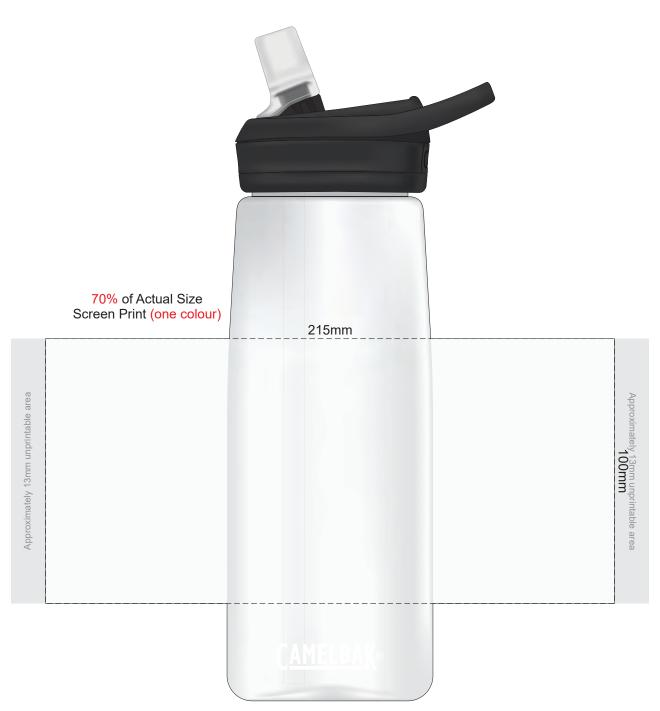
A 2-3mm tolerance is expected for alignment of the printed artwork and the CamelBak logo. Please note that there is a seam on the product that may run through the artwork. These seams are produced in the manufacturing process and are unavoidable.
