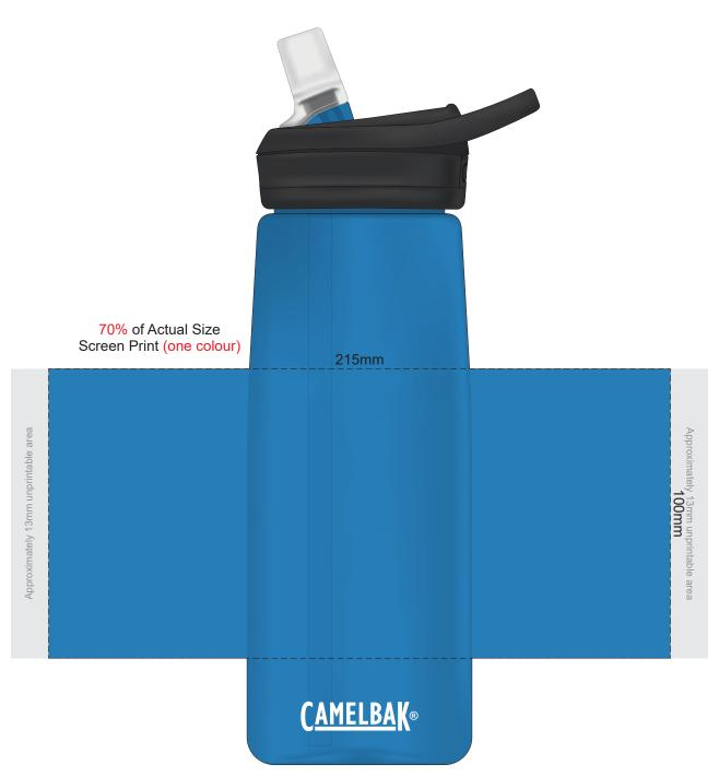
A 2-3mm tolerance is expected for alignment of the printed artwork and the CamelBak logo. Please note that there is a seam on the product that may run through the artwork. These seams are produced in the manufacturing process and are unavoidable.
